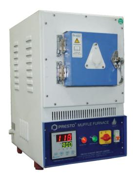
**Muffle Furnace** is a unique test cabinet designed to detect the percentage of ash content in a particular test specimen like rubber, elastomers. It is Bench top model and is used to evaluate the amount of inorganic compound in a test material.
